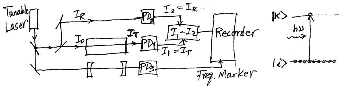
We split laser into three parts: one for absorption by the sample, one for reference beam of intensity, and the third for going through spectrum analyzer for frequency marker.
