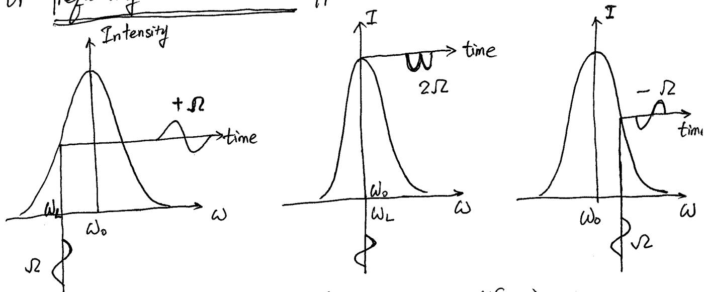
In phase-sensitive detection (lock-in amplifier)
