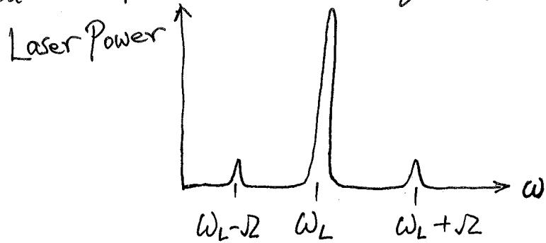
Three frequencies  $\omega_L \pm \Delta\omega$ ,  $\omega_L$  interact with the sample and we detect the overall effect.
