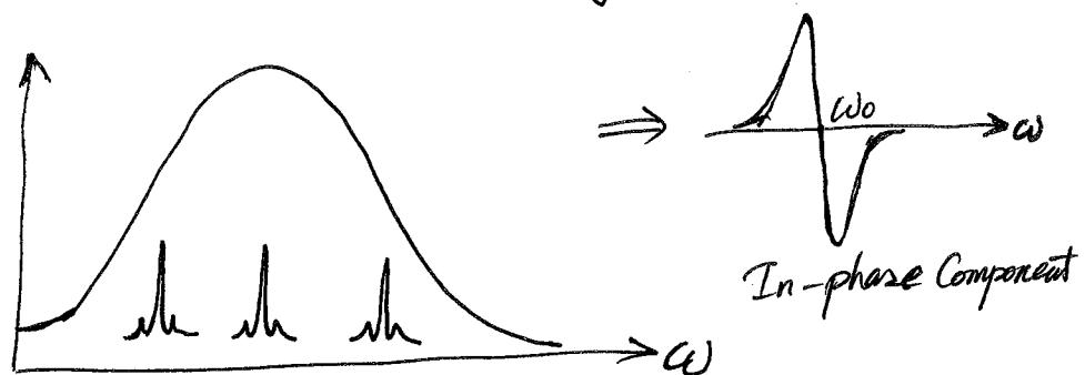
By adjusting the phase between the reference and signal, the lock-in output is the first derivative of the absorption line (in-phase component,  $\cos \sqrt{\omega} t$ ) or to the 2nd derivative of the dispersion ( $\sin \sqrt{\omega} t$ ).
