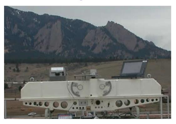
NOAA Dobson Spectrometer to measure ozone from the ground
