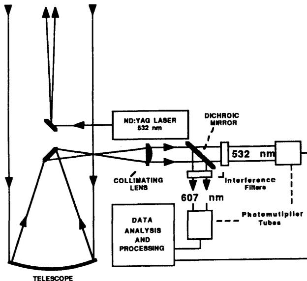
Fig. 1. Schematic diagram of the Raman-Rayleigh lidar.
