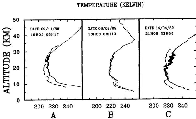
Fig. 3. Lidar temperature profiles compared with the corresponding balloon sounding obtained on (A) 09/11/88, 19H15; (B) 09/02/89, 07H30, (C) 14/04/89, 00H00.
