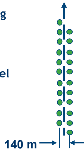
2 beams from 2 lasers or w/ a DOE
