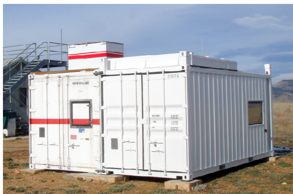
Figure 6. Mobile lidar laboratory consisting of two containers that host the MRI Fe Doppler lidar for mobile deployment.
