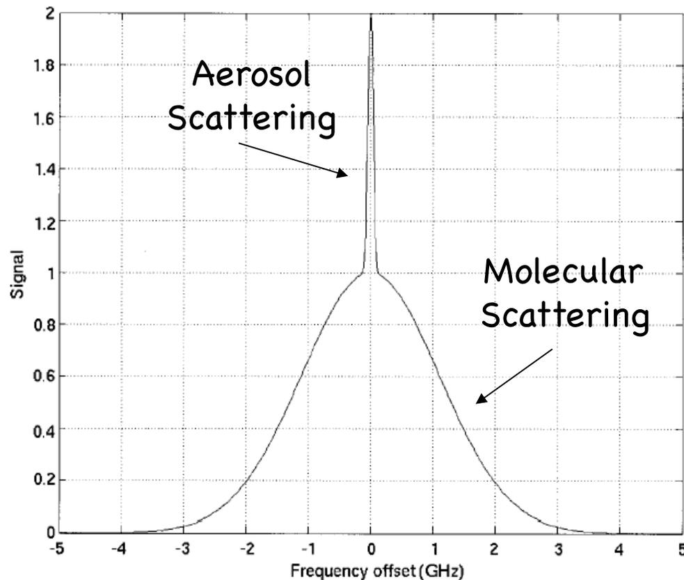
**Fig. 5.1.** Spectral profile of backscattering from a mixture of molecules and aerosols for a temperature of 300 K. The spectral width of the narrow aerosol return is normally determined by the line width of the transmitting laser.
