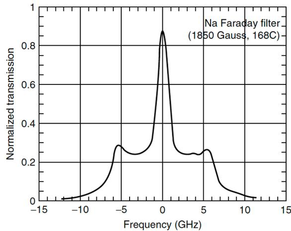
**Figure 5.16** Normalized transmission curve of a CSU Na lidar Faraday filter. (From Arnold, K.S., and She, C.Y., *Contemp. Phys.*, 44, 35–49, 2003. With permission.)
