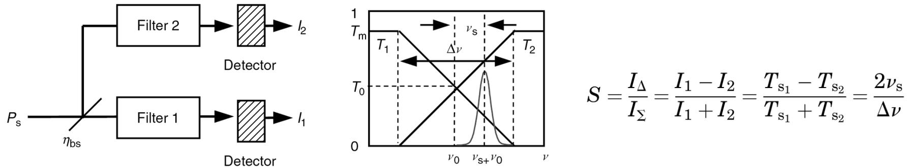
**Figure 7.32** Double-edge functional diagram and filter transmission.
