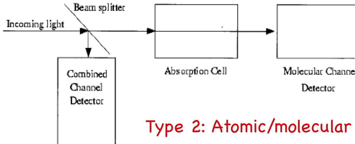
Atomic or molecular absorption block the aerosol scattering
