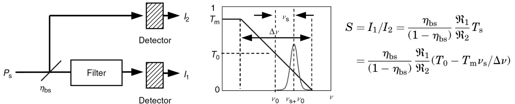
**Figure 7.31** Single-edge functional diagram and filter transmission.
