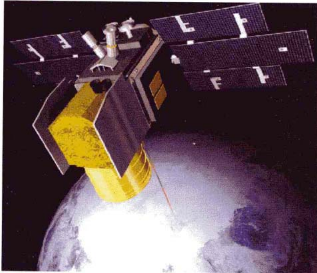
Fig. 13.23. An artist's rendition of the ICESat spacecraft with the GLAS instrument onboard. The 1064 nm and 532 nm laser pulses are shown probing the Earth's atmosphere and polar ice thickness changes. (Courtesy of S.P. Palm.)
