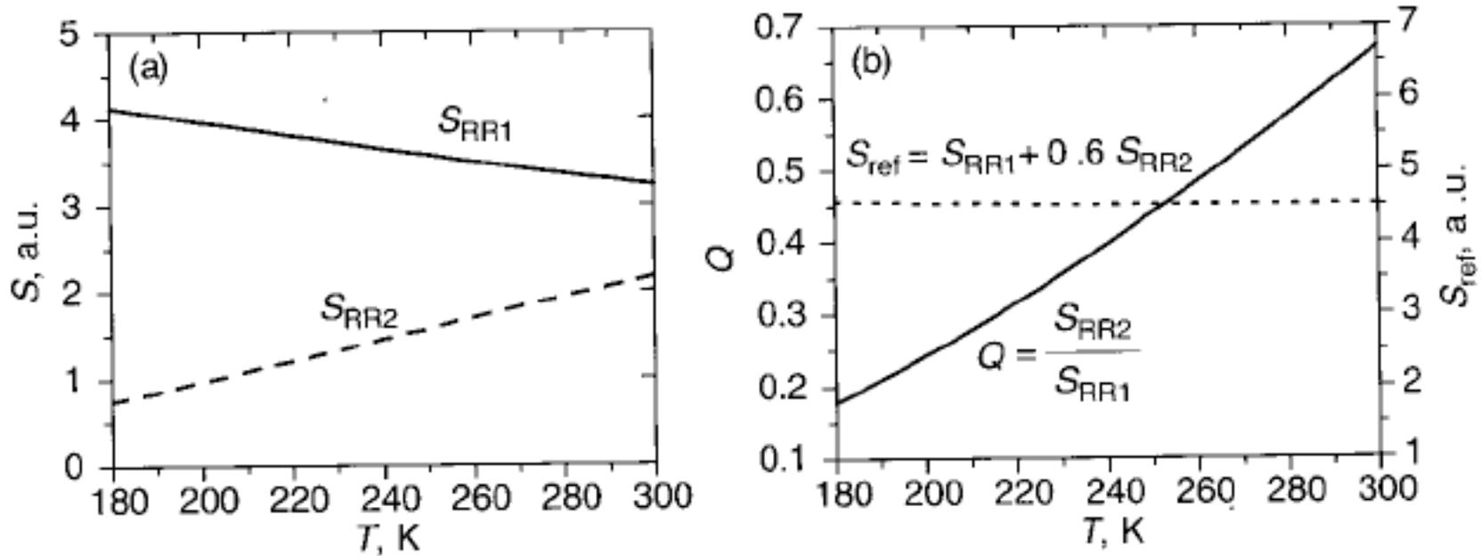
$$Q(T) = \frac{\sum_{i=O_2, N_2} \sum_{J_i} \tau_{RR2}(J_i) \eta_i \left( \frac{d\sigma}{d\Omega} \right)_{\pi}^{RR,i}(J_i)}{\sum_{i=O_2, N_2} \sum_{J_i} \tau_{RR1}(J_i) \eta_i \left( \frac{d\sigma}{d\Omega} \right)_{\pi}^{RR,i}(J_i)}$$
