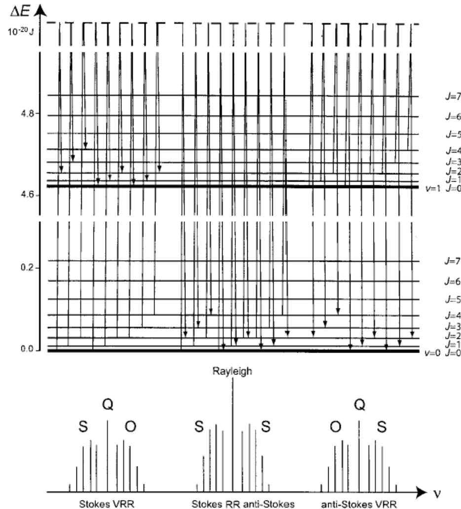
**Fig. 9.1.** Vibration–rotation energy levels of the N<sub>2</sub> molecule, Raman transitions, and resulting spectrum.
