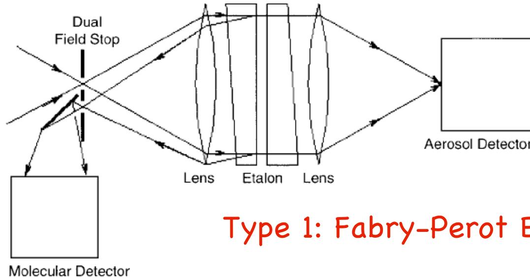
1. Aerosol scattering pass the transmission band
