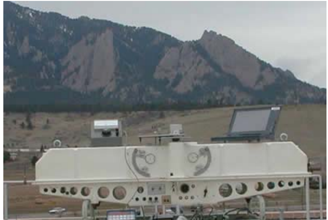
NOAA Dobson Spectrometer to measure ozone from the ground
